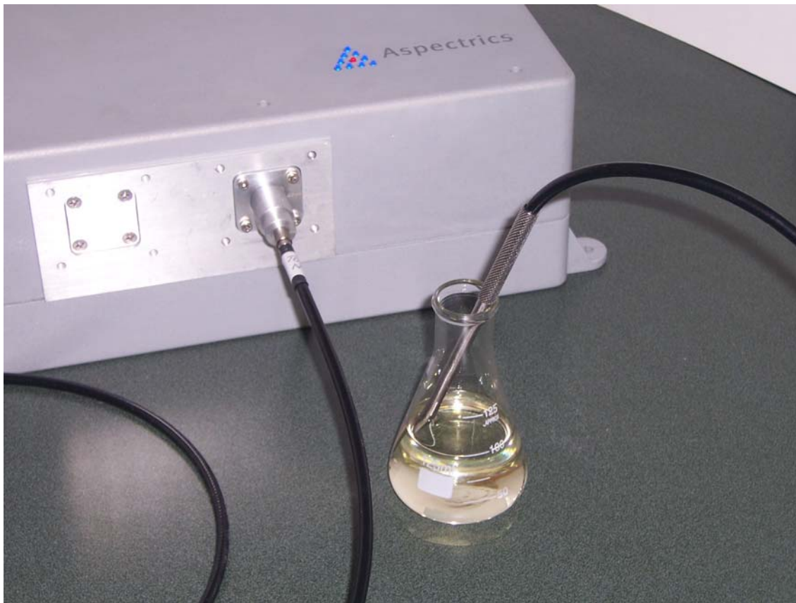
Figure 4: Aspectrics MC2750 EP-NIR spectrometer with an extended range transmission dip probe (600 microns polyimide) 2 mm pathlength.
