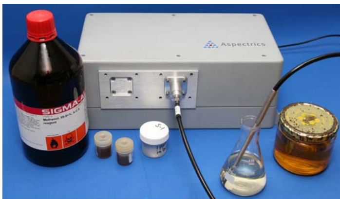
Fig. 1: EP-NIR MC2750 with dip probe and various samples (methanol, glycerin and actual ASTM 6751 compliant biodiesel samples.)
